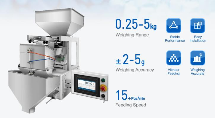
LF-5K is a linear feeder for granular materials and some powder materials. The vibratory feeding mechanism achieves multi-stage feeding. The pneumatic cylinder drives fast discharging. LF-5K linear feeder has a wide weighing range with high speed and high precision, which can be widely used in quantitative packaging machinery of grain, feed, chemical, rubber and plastic industries.
